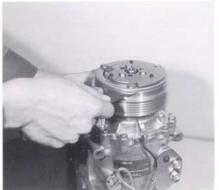
Fig 10. Air Gap Adjustment
