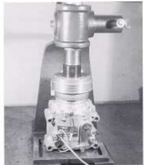
Fig 7. Installation of Clutch Rotor
