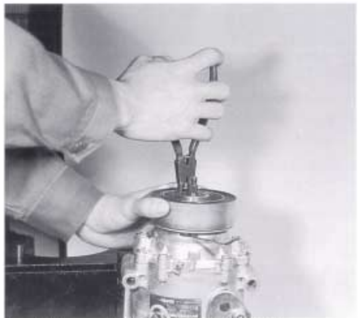
Fig 5. Removal of Clutch Coil Assembly
