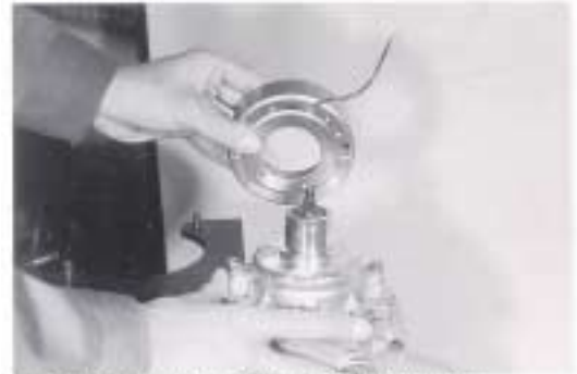
Fig 6. Installation of Clutch Coil Assembly
