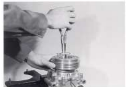
Fig 3. Removal of Snap Ring
