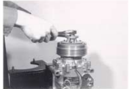
Fig 1. Removal of Armature Fixing Nut
