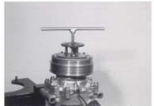
Fig 2. Removing Clutch Armature Assembly
