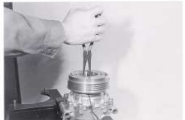
Fig 8. Installation of Snap Ring
